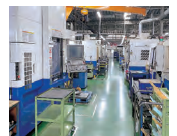
Small batch production line for torque converters
